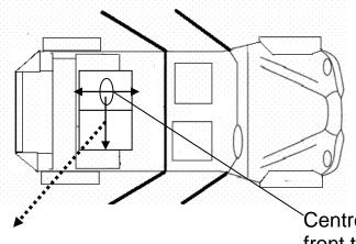
Centre point of seat front to rear from which to measure width of rear seat
